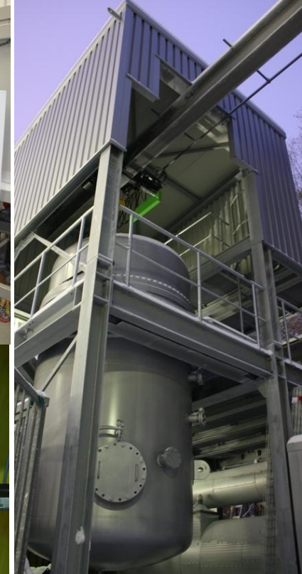
Test rig "HOTREG" for high-temperature regenerator storage at DLR Stuttgart
